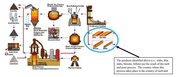
**First (Semifinished) Mill Test Certificate:** The above diagram shows the manufacture of steel in its first solid, semifinished, state. The country where steel is <u>originally</u> produced in either an Electric Arc Furnace or a Basic Oxygen Furnace is the <u>country of melt and pour</u>. A mill test certificate should display the chemistry, the mill location, and the heat number. It may also display the semifinished product type.
